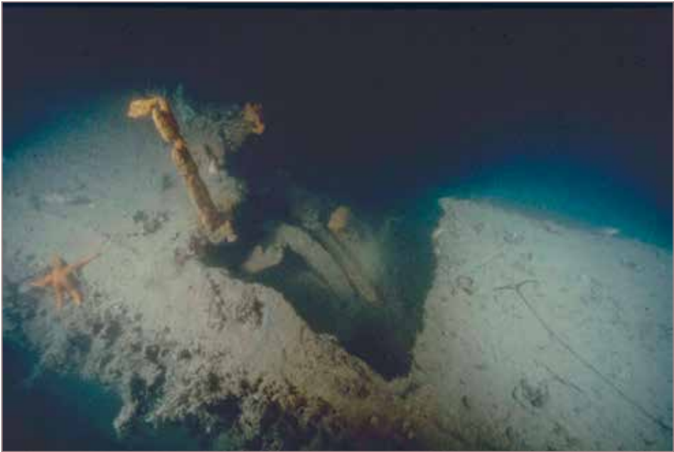
The distinctive ramp in the forward casing of AE2—a feature only of the early “Group 1” E-Class submarines (E1–E9, AE1 and AE2). A wooden lid once covered the ramp to give access to the anchor winch (Photo Mark Spencer).
